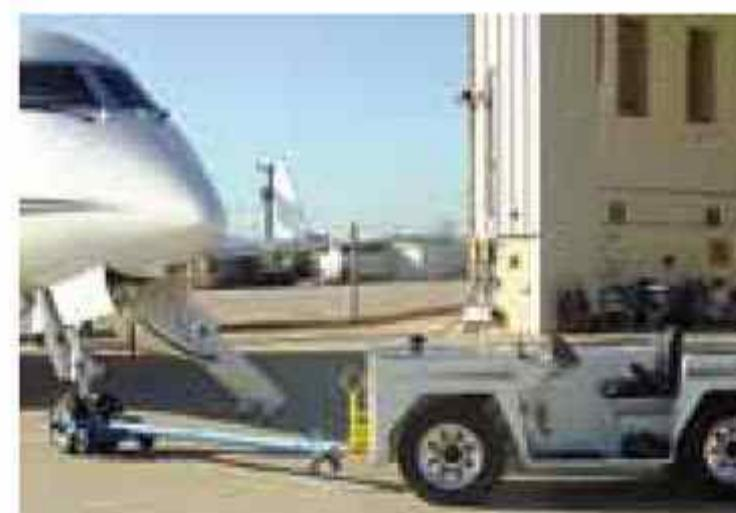
Eagle Tugs, All Wheel Drive Aircraft Tractors. Engineered to meet the needs of regional airlines, corporate flight departments, fixed base operators and military flight operations, the Eagle TT series all wheel drive aircraft tractor packs a significant amount of value into a small package. Whether you're moving Gulfstreams, ERJs, CRJs, C130s or a Blackhawk Helicopter, Eagle has a tractor that will suit your needs in any environment.
